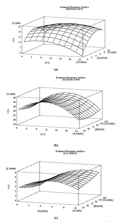
$\label{eq:Fig. 5.} \textbf{Fig. 5.} \ \text{Response surfaces estimated from the central composite design by plotting (a) [Ce (IV)] vs. [Na_2SO_3], (b) \\ \hspace{0.5cm} [Ce (IV)] \ vs. \ [H_2SO_4], (c) \ [Na_2SO_3] \ vs. \ [H_2SO_4].$
