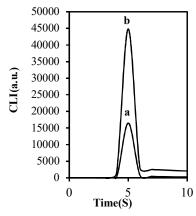
Fig. 2. Kinetic curve for Ce(IV)-Na<sub>2</sub>SO<sub>3</sub> CL system, (a) alone, (b) in the presence of methamphetamine. Conditions: Ce(VI), 1.25 × 10<sup>-3</sup> M; Na<sub>2</sub>SO<sub>3</sub>, 7.5 × 10<sup>-4</sup> M; H<sub>2</sub>SO<sub>4</sub>, 1.25 × 10<sup>-2</sup> M and methamphetamine, 0.3 μg/mL.
