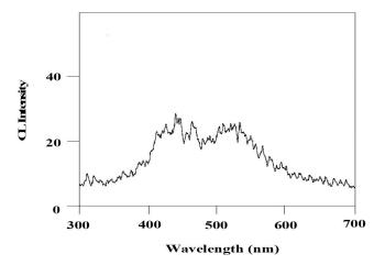
Fig. 3. CL spectrum of Ce(IV)-Na<sub>2</sub>SO<sub>3</sub> system (a) in the absence and (b) presence of methamphetamine obtained with continuous flow of reagents: Ce(IV),  $2.5 \times 10^{-3}\,$  M and H<sub>2</sub>SO<sub>4</sub>,  $2.5 \times 10^{-2}\,$  M in one line and Na<sub>2</sub>SO<sub>3</sub>,  $1.5 \times 10^{-4}\,$  M with methamphetamine (20 µg/mL) in other line.
